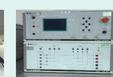
Fully automatic lightning strike surge tester
